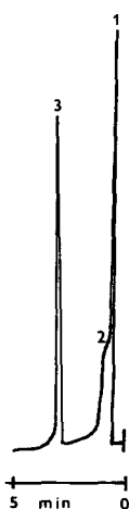
Fig. 1. Chromatography of distilled water containing 0.01% of each alcohol on an Apiezon L glass column (2.5 m \times 4 mm I.D.) at 97°C. Peaks: 1 = methanol; 2 = water; 3 = and n -butanol.
